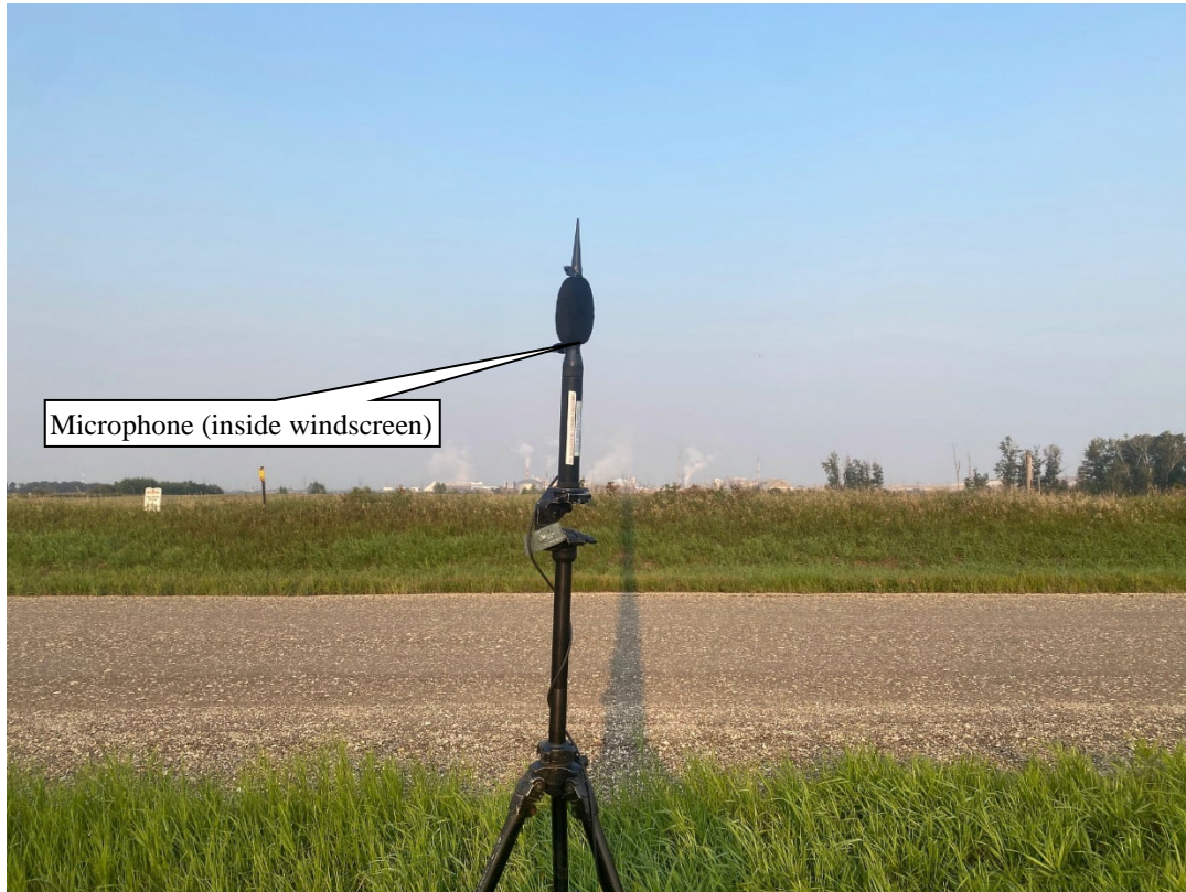
Figure 8. Noise Monitor #6 (With Weather Monitor)
